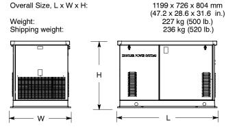
NOTE: This drawing is provided for reference only and should not be used for planning installation. Contact your local distributor for more detailed information.
