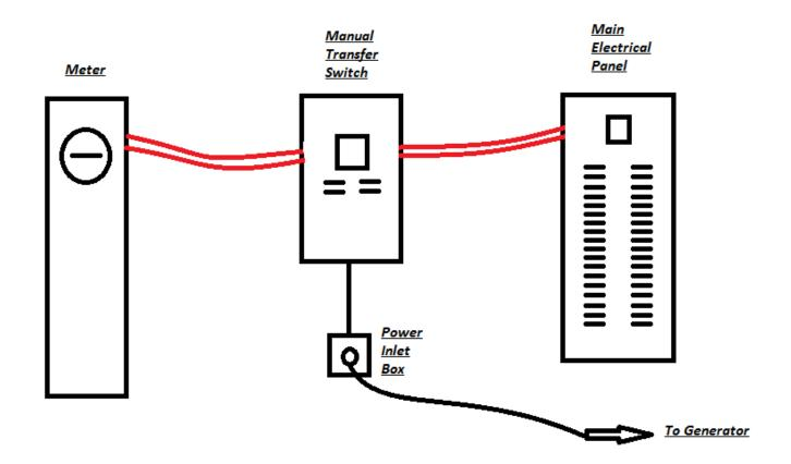
Note: Equipment should be installed by a certified electrician to meet all local codes.
