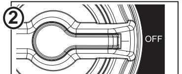
2. Turn the fuel selector switch to **OFF** and stop the flow of fuel by cylinder valve or the valve on the natural gas hose.
