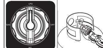
3. For propane, rotate the fuel selector switch to **NG** (natural gas) and open the natural gas valve.
